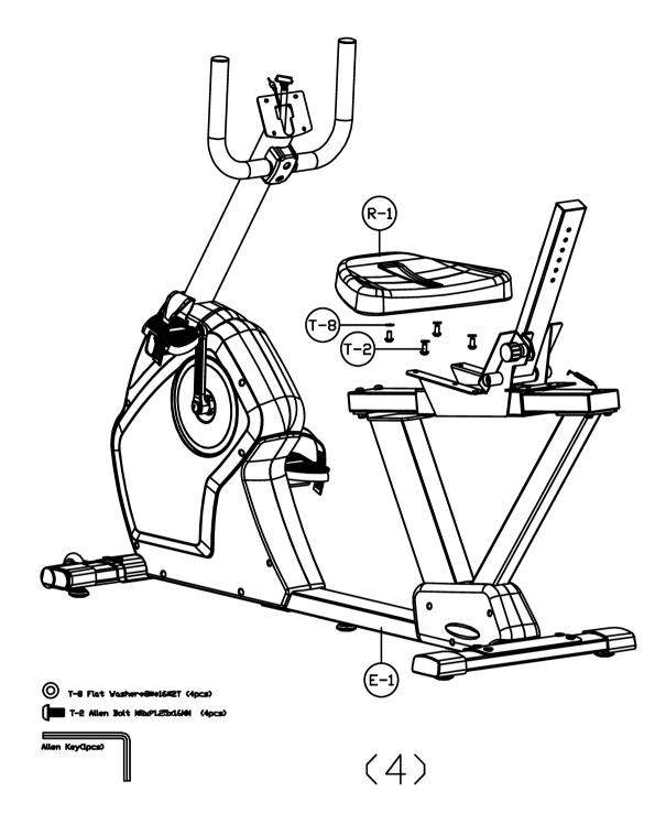
1. Assemble the Seat (R-1) to the Seat Slider with 4 Flat Washers (T-8) and 4 Screws (T-2)
