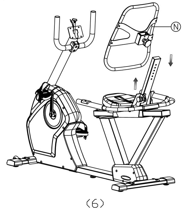
1. Slide Back Rest (N) through Back Rest Slider (M-1)
